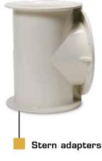
Also manufactured from fully isophtalic resin, Max Power's range of stern adaptors are SMC moulded (sheet moulding compound) in a male  $\neq$  female steel mould. This ensures perfect resin fibre ratio and exceptional reproduction of form.
