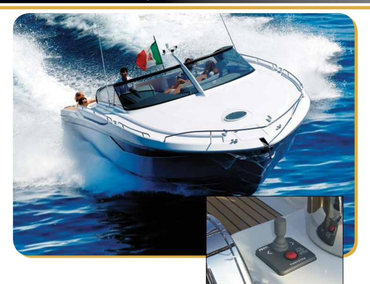
All control panels are specially designed for use with Max Power's complete range of tunnel and retractable thrusters. Fitted using a simple hole saw cut-out, panels are easy to install and benefit from a simple and easily replaceable weatherproof clip-on cover. Each panel is complete with both male and female connectors using a reusable connection system.
