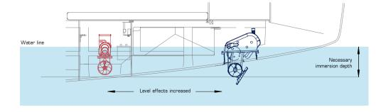
Installed further forward (or aft) in the hull than is possible with a tunnel thruster, retractable units offer a far better turning moment on the yacht thus producing greater manoeuvrability.
