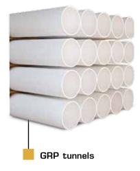
Manufactured from fully isophtalic resin and pre-gel coated, Max Power's high quality tunnels have the added advantage of a first coat of matt before being filament wound. Cutting and drilling can therefore be carried out without the risk of damaging the gel coat on the inside surface of the tunnel.
