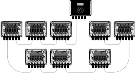
The figure shows a typical installation system using <u>only 1 main control module CAN Bus trunk</u> Any combination of the systems shown above can be envisaged.
